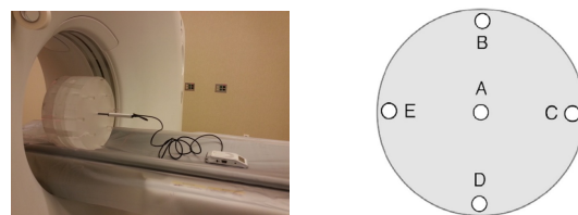
(a) Phantom image (b) Axial view of measurement position Fig. 1 Dose measurement using of PMMA phantom
