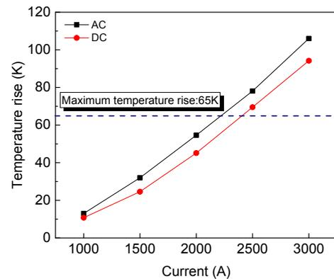
**Fig. 11.** Comparison of temperature rises of AC-GIL and DC-GIL conductors with variation of the load current
