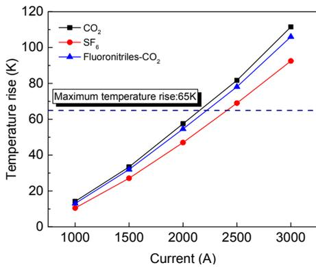
**Fig. 8.** Relationship between load current and the temperature rise in the GIL conductor
