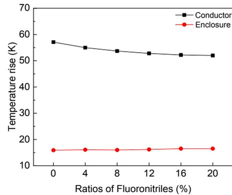
Fig. 6. Relationship between the temperature rise of the GIL and the proportion of Fluoronitriles gas used
