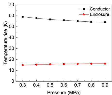
Fig. 7. Relationship between gas pressure and GIL temperature rise
