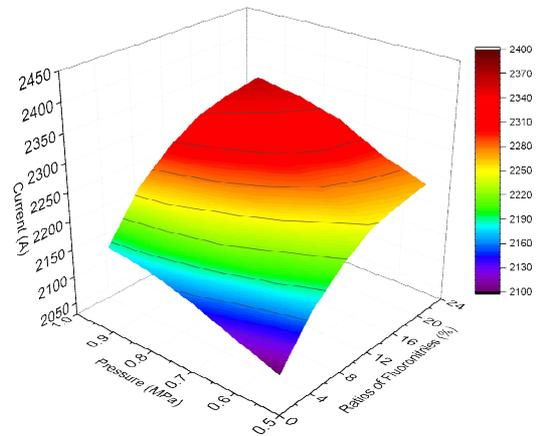
**Fig. 9.** Relationship among the current-carrying capacity of the GIL conductors, the gas pressure and the ratio of the Fluoronitriles
