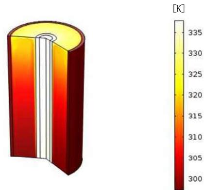
**Fig. 10.** Temperature distribution of DC GIL filled with Fluoronitriles-CO<sub>2</sub> mixture
