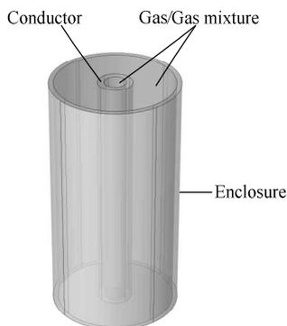
Fig. 1. Geometric model of the GIL
