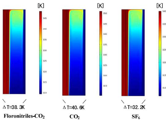
Fig. 5. Temperature distributions of GILs filled with the Fluoronitriles-CO<sub>2</sub> mixture, CO<sub>2</sub>, and SF<sub>6</sub>
