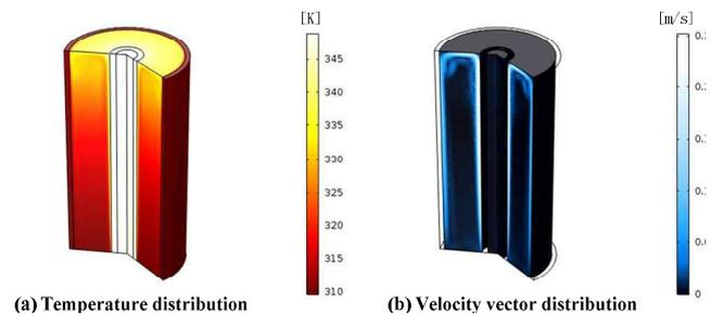
**Fig. 4.** Temperature and gas flow velocity distributions of the GIL under steady state conditions
