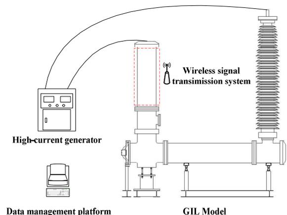
Fig. 3. Temperature rise test platform for the GIL
