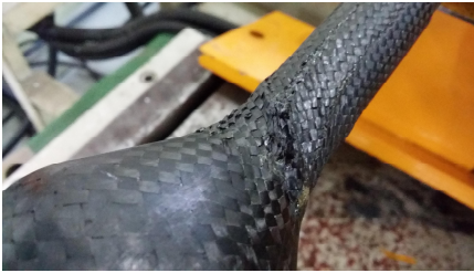
Fig. 2 Fractography of CFRP Tube
