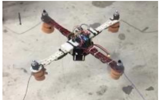
Fig 11. 2-axis Control Test
