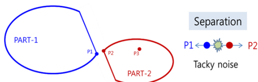
Fig. 4 Principle of separation noise.
