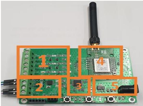
Fig. 6. Implementation of Controller for Dew Condensation Prevention of Distributing Board.
