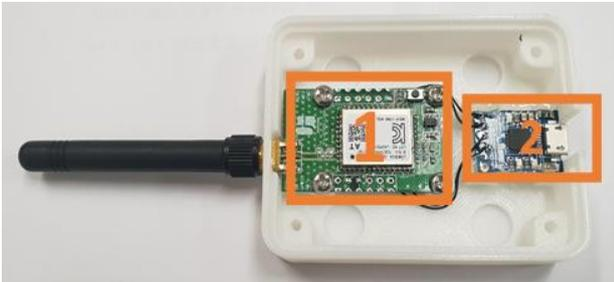
Fig. 9. Implementation of Monitoring Receiver for Dew Condensation Prevention of Distributing Board.
