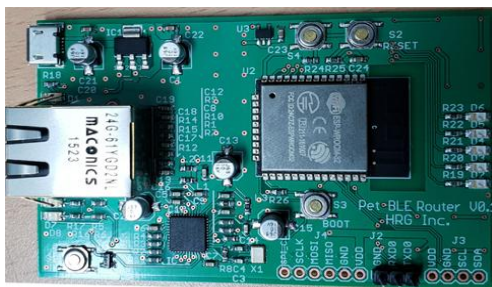
Fig. 8. The implemented Bluetooth router
