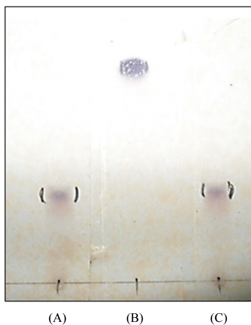
Fig. 8. TLC analysis of purified siderophore. (A) siderophore produced from Acinetobacter sp. B-W grown in medium containing glutamic acid as both carbon and nitrogen sources at 28°C (B) 0.5% 2, 3-Dihydroxybenzoic acid, (C) siderophore produced from transformant E. coli DH5a. TLC F254 silica gel plate in combination with a mixture of butanol : acetic acid : water (12 : 3 : 5, v/v/v) as mobile phase was used. Plate was sprayed with 1% ferric ammonium citrate and then with potassium ferricyanide.
