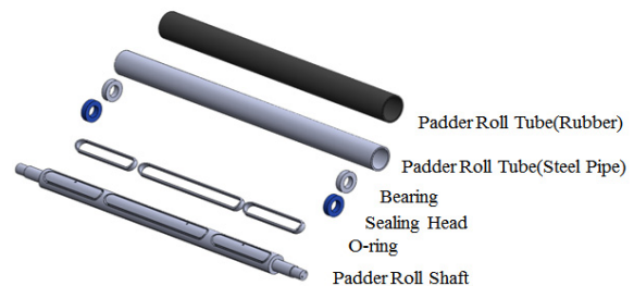
Fig. 1 Structure of Padder Roll
