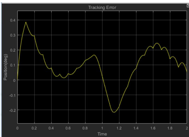
Fig. 7 Tracking error of left ankle joint in sagittal plane when traditional PID control is implemented without TDC
