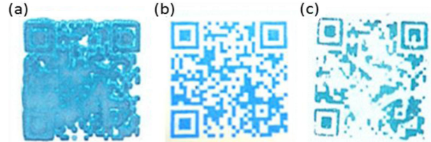
Fig. 2. Silk screen printing performance with respect to screen size. (a): 200 mesh, (b): 250 mesh, (c): 350 mesh. Formulation 2 was used. TTI was printed in QR code image.
