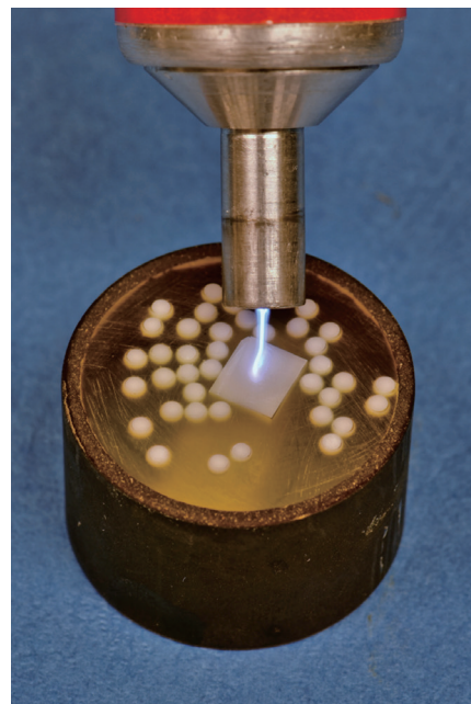
Fig. 1. Plasma activation of the surface of an embedded zirconia specimen previous to adhesive treatment.
