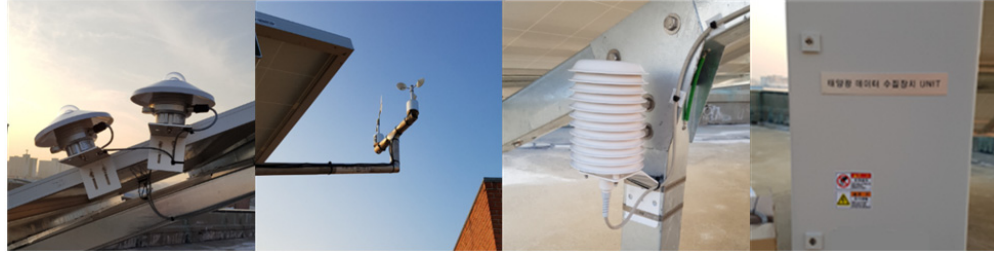
Fig. 2 H University meteorological monitoring system (solar pyranometer, weather vane and anemometer, thermo-hygrometer, data collecting device)
