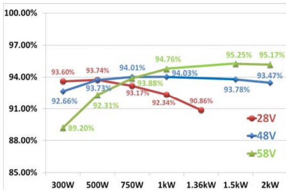
Fig. 13. Efficiency characteristics in the PM mode.
