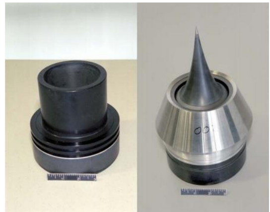
Fig. 4. Conventional conical nozzle(left) and aerospike nozzle(right) [21]
