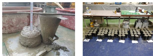
**Photo 1** Visual of slump and test specimens
