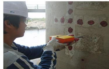
Fig. 2 Rebound hardness test
