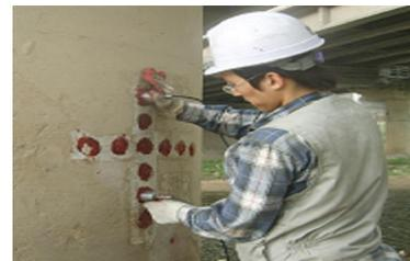
Fig. 3 Ultrasonic pulse velocity test
