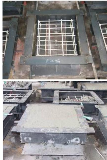
Fig. 3 Push-out specimen fabrication
