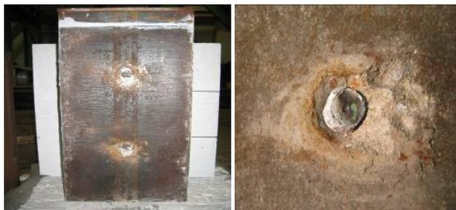
Fig. 6 Failure pattern of Push-out specimen
