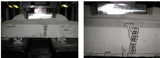
(a) No.14 : rail-seat section (b) Detail of cracks in No.14
