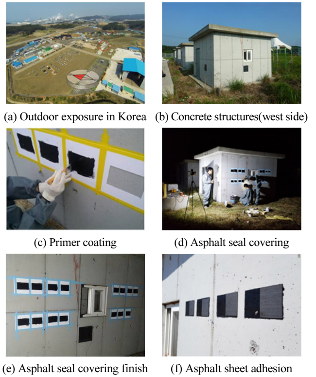
Photo 2 Experiments of vertical sagging down resistance at outdoor exposure
