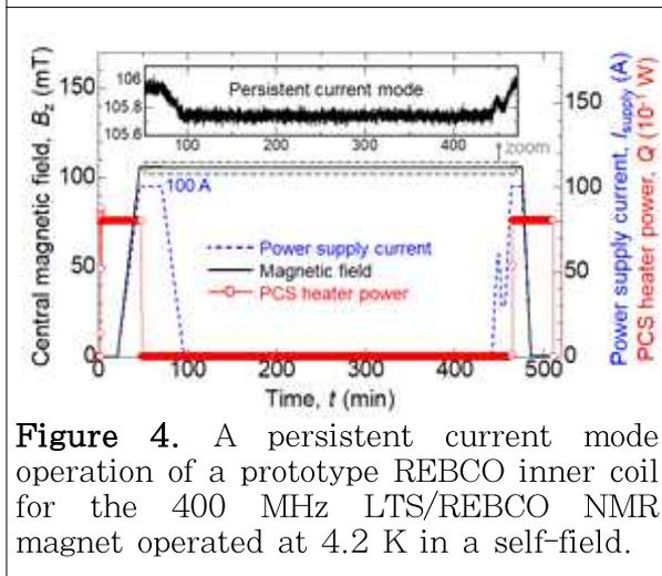
**Figure 4.** A persistent current mode operation of a prototype REBCO inner coil for the 400 MHz LTS/REBCO NMR magnet operated at 4.2 K in a self-field.
