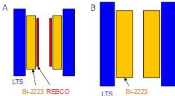
**Figure. 1.** Two schematics of the coil cross section of 1.3 GHz NMR magnet (not to scale).
