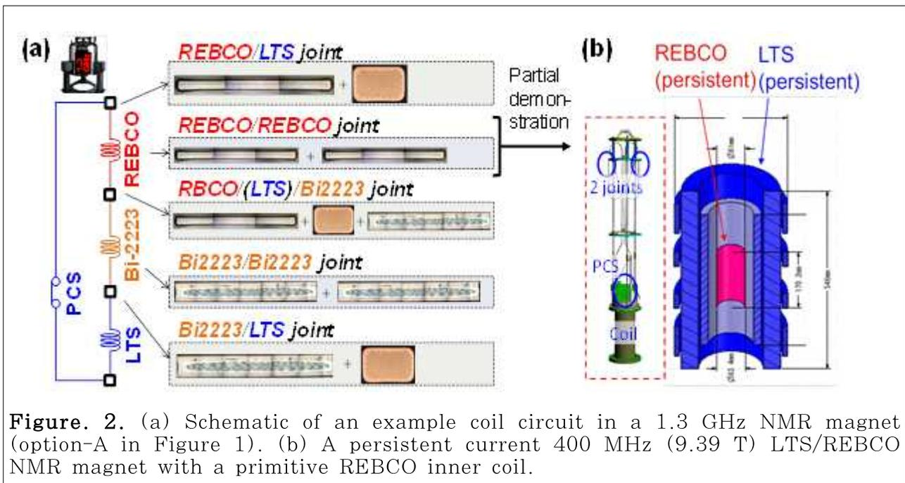
**Figure. 2.** (a) Schematic of an example coil circuit in a 1.3 GHz NMR magnet (option-A in Figure 1). (b) A persistent current 400 MHz (9.39 T) LTS/REBCO NMR magnet with a primitive REBCO inner coil.
