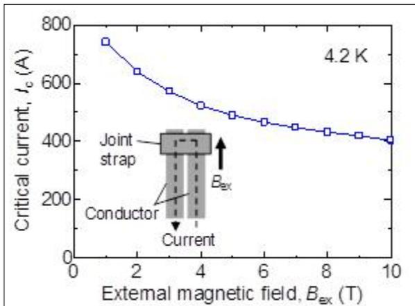
**Figure 3.**  $I_c$ – $B$  characteristics of a joint sample of REBCO wires in magnetic fields parallel to the joint plane measured at 4.2 K.  $I_c$  was determined with a voltage criterion of 1  $\mu$ V.
