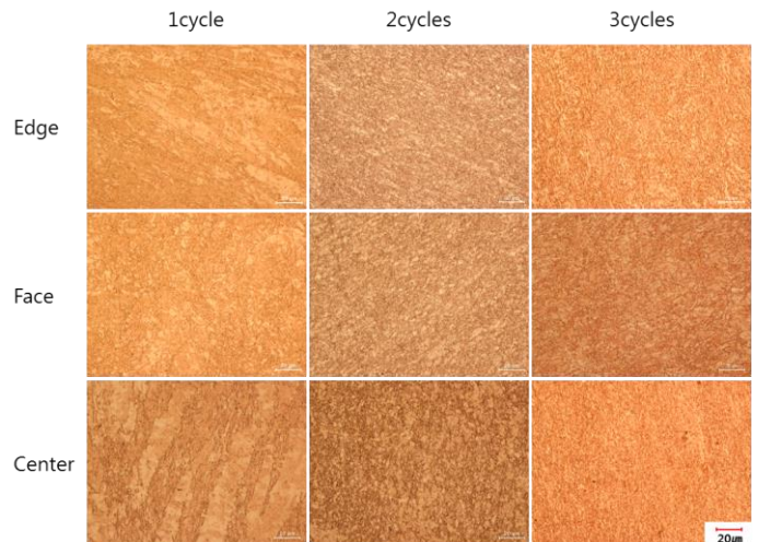
Fig. 5 Microstructure of MADF processed OFC
