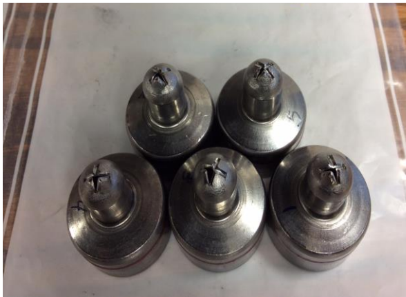
Fig. 12 Prototype Samples After Pressurizing Burst Test
