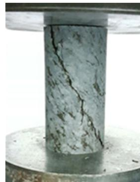
Fig. 4. Universal test machine for measuring direct compressive strength
