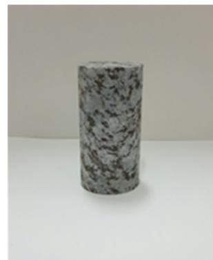
Fig. 1. A specimen of granitic gneiss
