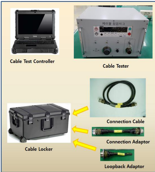
Fig. 17. Shape of the Automatic cable assembly test system
