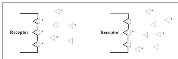
Figure 1. Schematic Drawing of Receptor Imaging with High Molar Activity (left) and Low Molar Activity (right) Radiopharmaceuticals. Triangle Indicates Compound and an Asterisk Indicates Radioisotope.
