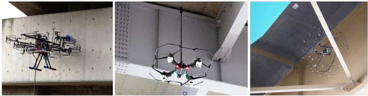
〈Fig. 8〉 Various drones available for visual inspection of spatial structures
