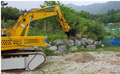
Fig. 12 Bucket's contact for topographical recognition
