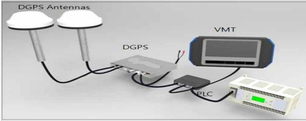
Fig. 5 Yard automation equipment configuration
