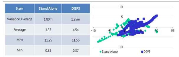
Fig. 12 DGPS Test result(Container packed Yard)
