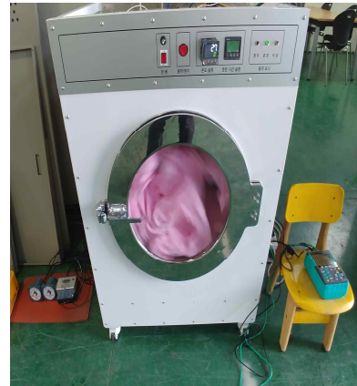
Fig. 1 The Dryer Fabricated with a Heat Source Using Carbon Nanofiber Lamp
