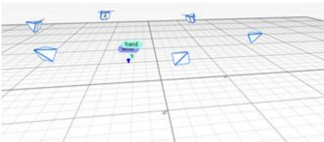
Fig. 2. Six cameras were set up 1.8 meters above the ground forming a 2.5m-diameter circle (above). Then, the test environment was demonstrated on Motive
