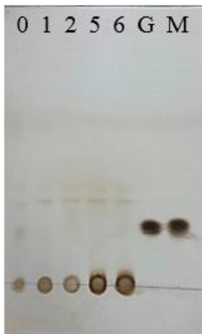
Figure 3. TLC development of KMOS derived from the hydrolysis of KM. Bacillus N3 was incubated in 200 ml medium consisting of 0.5 % KM in 1/20 diluted LB for 7 days at 30 °C. Culture supernatant was collected and heated at 100 °C for 5min. Then, KMOS in the supernatant derived from the time-dependent hydrolysis were developed on TLC plate. G: Galactose; M: Mannose; 0: KMOS-0; 1: KMOS-1; 2: KMOS-2; 5: KMOS-5; 6: KMOS-6. Numbers indicate the time (day) of incubation as shown in Scheme 1, as shown in the Materials and Methods section.
