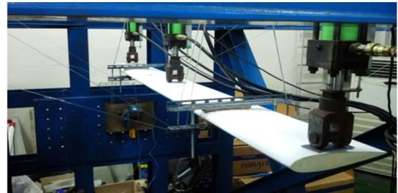
**Fig. 12** Structural test of blade
