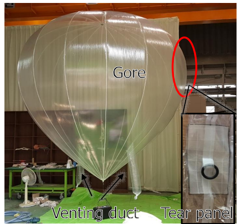
Fig. 7. Manufactured configuration of the envelope [Class 10 km / 3 kg]
