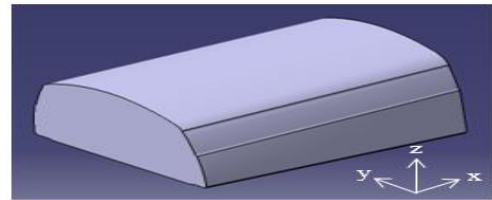
Fig. 3. Simplified Conformal Fuel Tank CATIA Model
