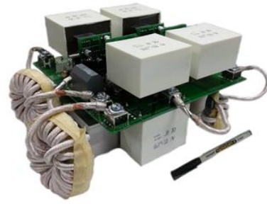
Fig. 8. Photograph of the proposed converter 2-kW prototype.
