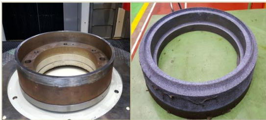
Fig. 4 Specimen and grinding wheel of curvic coupling tooth
