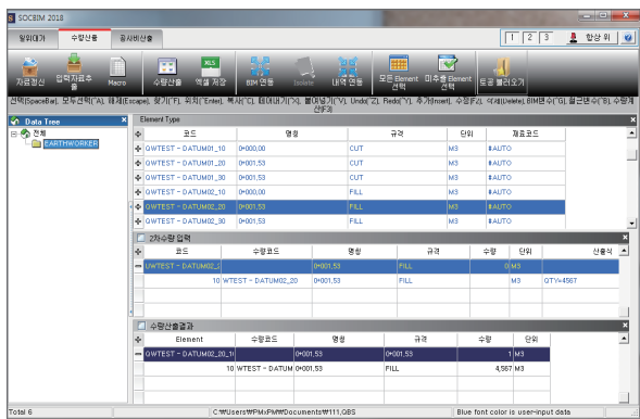
Figure 6. Parametric Quantity Take-Off of Earthwork by Solid Models
