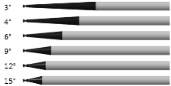
Fig. 8 Configuration of supercavitating bodies with various slant angles
