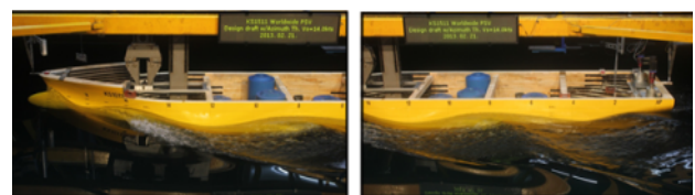
Fig. 7 Resistance test (initial hull form A, design draft at 14 knots)
