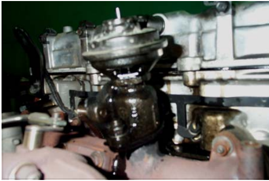
Fig. 2. Oil leakage example of EGR Valve assembling parts.
