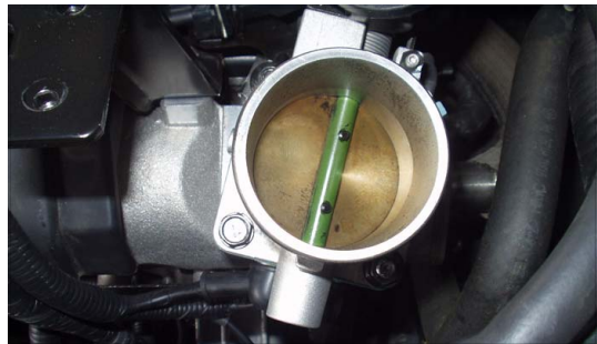
Fig. 4. Sticking example of throttle flap inflow the air.
