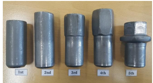
Fig. 1 5-step sequence for forming a wheel nut
