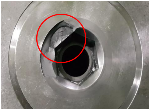
Fig. 5 Fractured area of insert ring of 5th die
