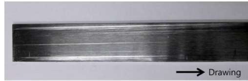
Fig.4 Galling at specimen during friction test(Room temperature, Contact pressure: 1.5Mpa)
