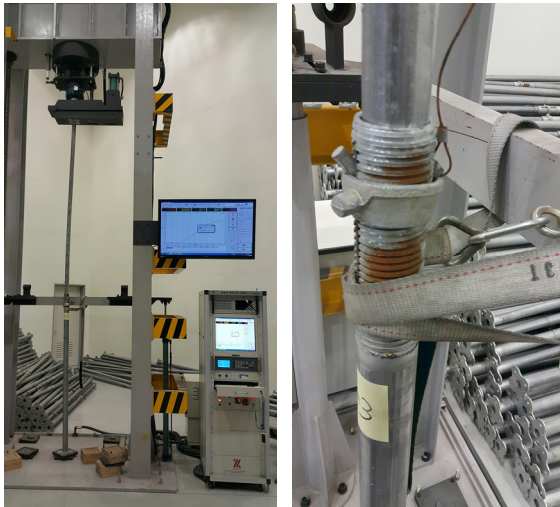
Fig. 10. Pipe support failure type due to compressive load(1)
