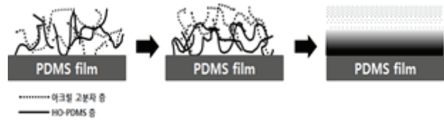
Figure 6. Schematic presentation for microphase-separation occurring surface-modifier-coated PDMS film.
