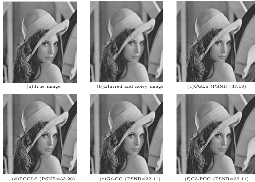
Fig. 1. Lena image for Disk blur with reflexive BC ((c, d, e, f): restored images for Case 2 of D ).
