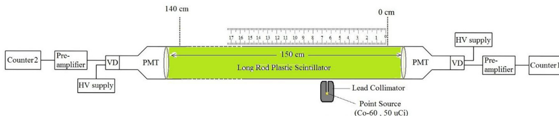
Fig. 1. The arrangement of the source and nuclear electronic system (experimental set-up).
