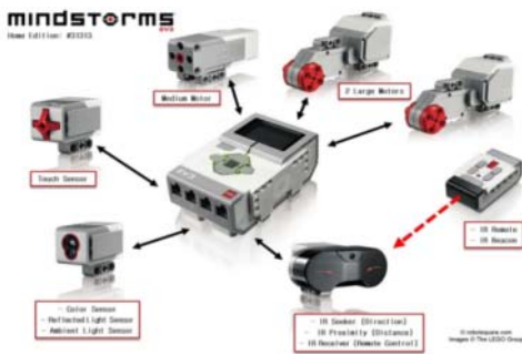
Figure 1. Motors and Sensors connected to ev3 (robotsquare.com, The LEGO Groups)
