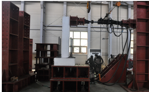
Fig. 11. Hybrid Simulation setup
