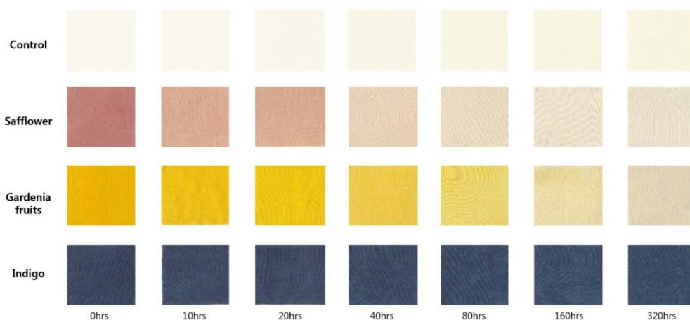
Figure 1. Color fading sequence of the samples. (a) safflower, (b) gardenia, (c) indigo.
